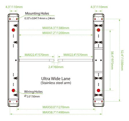
Note: When the lane width is 35.4 in - 47.2in (900mm - 1200mm), stainless steel barriers are required.
