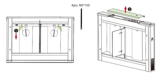
2. In the position shown below, use a Phillips screwdriver to unscrew the four fixing screws (round head Phillips screws with washers) of the authentication panel.
